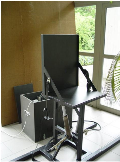
Figure 1. Tilt chair used for Subjective Postural Vertical assessment
