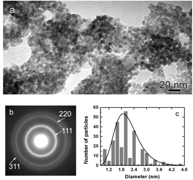
FIG. 2. (a) TEM image revealing the mesoporous morphology of the  $\text{cZnS:Mn}$  QDs sample. (b) The corresponding electron diffraction pattern indexed with the cubic (sphalerite)  $\text{ZnS}$  structure. (c) Histogram showing the size distribution of the  $\text{cZnS:Mn}$  crystallites.
