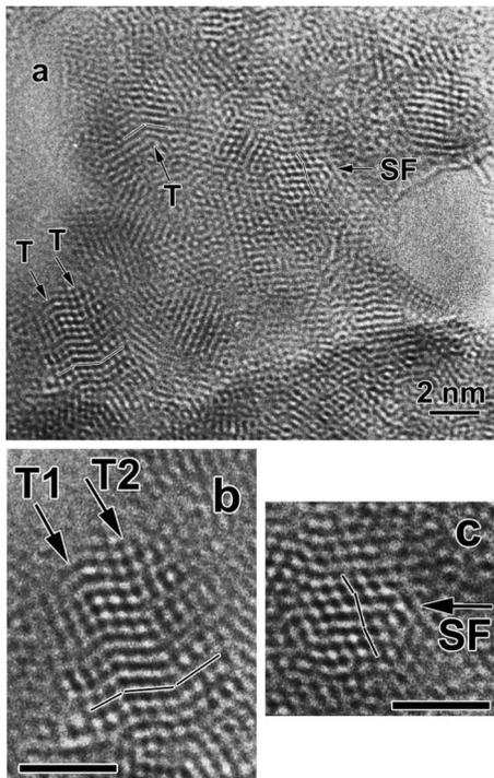
FIG. 3. (a) HRTEM image of the cZnS:Mn QDs sample revealing in some crystallites (marked by arrows) planar defects such as twin interfaces (t) and stacking faults (SF). (b) and (c) enlarged HRTEM images of crystallites oriented along the  $[110]$  zone axis showing the atomic structure of these defects. The black lines are drawn to guide the eye. Scale bars: 2 nm.
