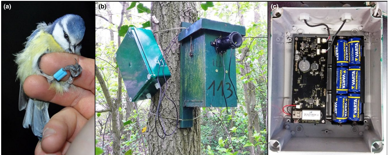
FIGURE 1 (a) An example of a PIT tag, here embedded in a leg band and attached to a blue tit. (b) Waterproof box containing the radio-frequency identification (RFID) logger mounted on a tree (left side) with antennas placed in front of the nest box opening. (c) Inner side of the RFID box, containing the battery holder, RFID data logger circuit, and a 1 GB memory stick for data storage and programming
