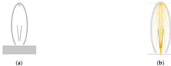
Figure 3. Visualisation of the optimised geometry and the related ray trajectories. (a) Optimised geometry according to simulations; (b) Ray trajectories according to ray-tracing simulation.
