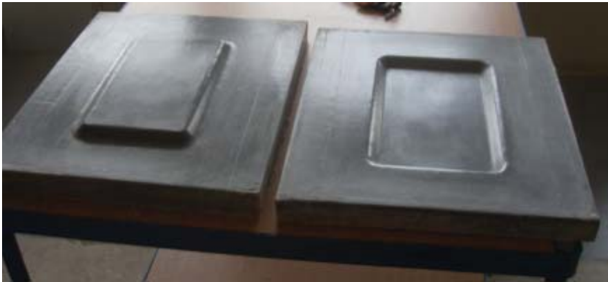
Figure 8. Matched die TRC mold
