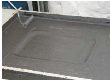
Figure 6. Workability of topcoat with AEROSIL and Dupont Alesta HR filler
