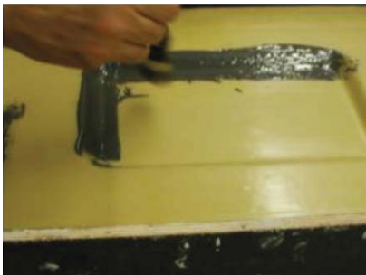
Figure 6. Workability of topcoat with AEROSIL and Dupont Alesta HR filler
