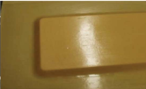
Figure 5(b). Master model covered with wax sheet
