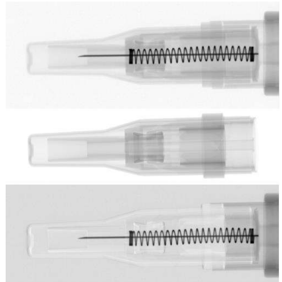
Figure 7: Simultaneous spectrum and 3D registration estimation with 108 energy bins of experimentally measured projection data. A single measured projection is shown (top) along with its corresponding 3D registered CAD projection (middle) and a difference image (bottom).
