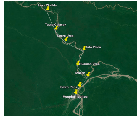
FIGURE 6: Schema of the rural Napo network, connecting several villages to the city of Iquitos using a set of linearly arranged point-to-point wireless links.
