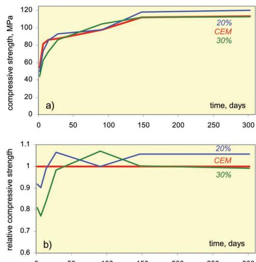
Fig. 10. Compressive strength and relative compressive strength of specimens with DRL WGP
