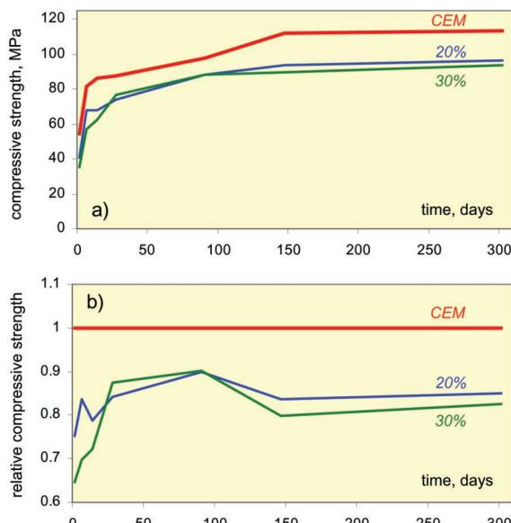
Fig. 6. Compressive strength and relative compressive strength of specimens with flint WGP
