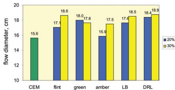
Fig. 3. Consistency tests results
