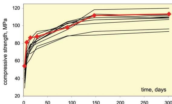
Fig. 5. Evolution of the compressive strength of the specimens stored under water
