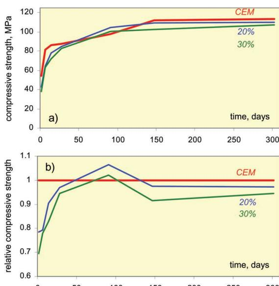
Fig. 7. Compressive strength and relative compressive strength of specimens with green WGP
