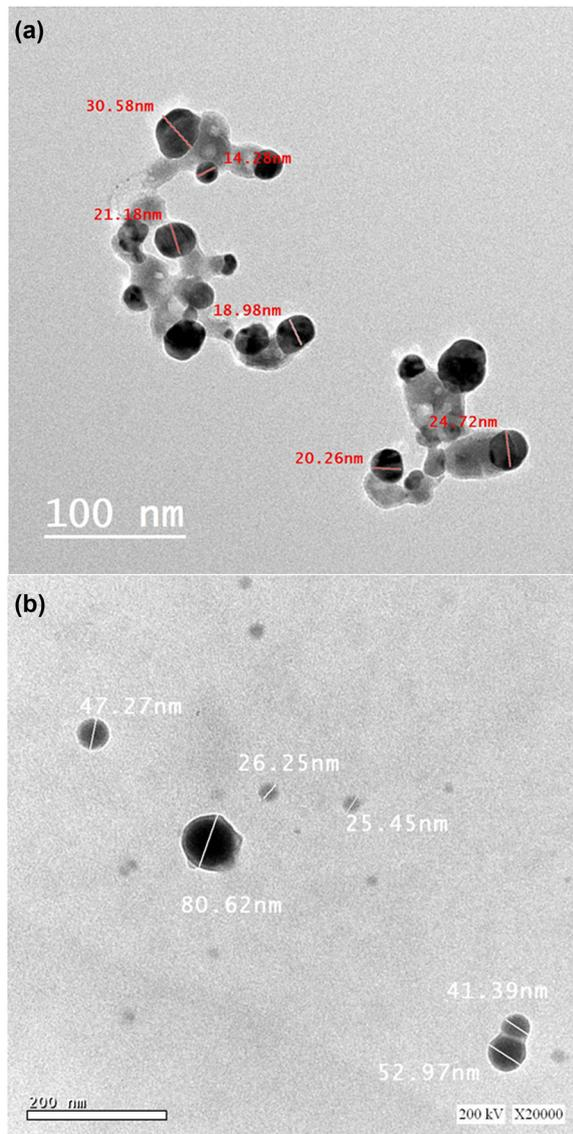
**Figure 3:** TEM images of biosynthesized AgNPs (a) and SeNPs (b).
