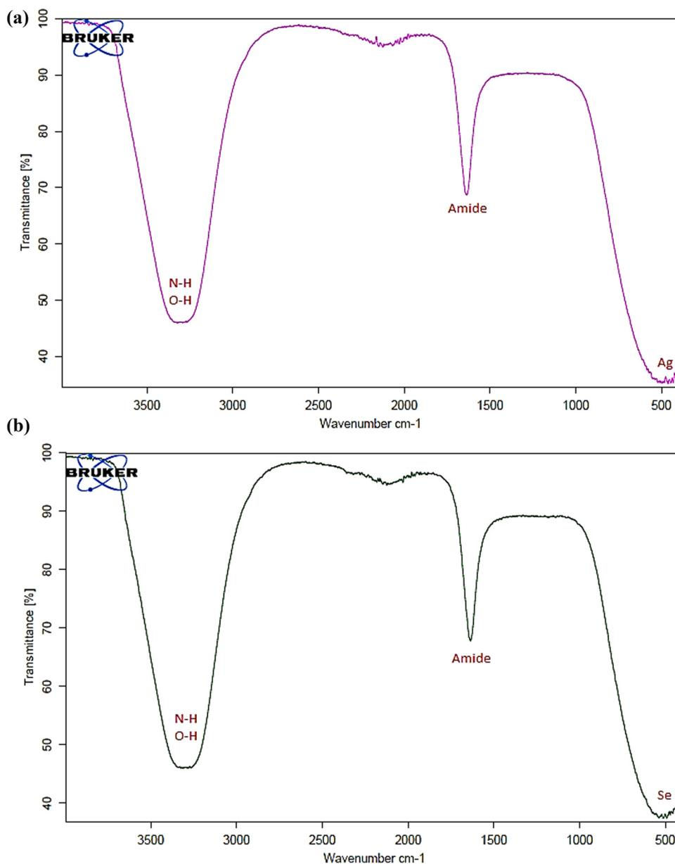
Figure 2: FTIR spectra of AgNPs (a) and SeNPs (b) produced by *T. viride*.
