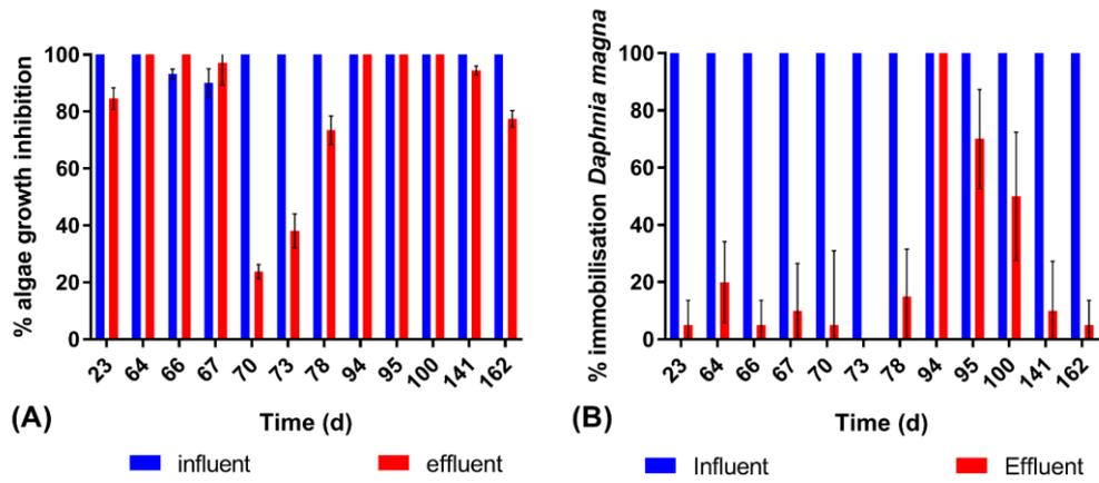
Figure 5: Effluent and influent ecotoxicity of different samples during the whole reactor operation tested with (A) *Pseudokirchneriella subcapitata* and (B) *Daphnia magna*.
