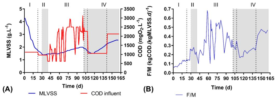
Figure 1: (A) MLVSS concentration and influent COD. (B) F/M ratio in the reactor during the whole operation period. (Vertical dotted line represents a switch to a new influent batch) (note: in stage III, a new influent batch was used every day)
