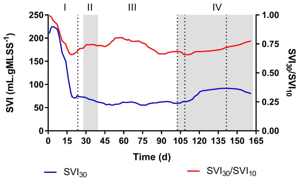
Figure 2: Evolution of the  $SVI_{30}$  and  $SVI_{30}/SVI_{10}$  during the whole operation period. (Vertical dotted line represents a switch to a new influent batch) (note: in stage III, a new influent batch was used every day)
