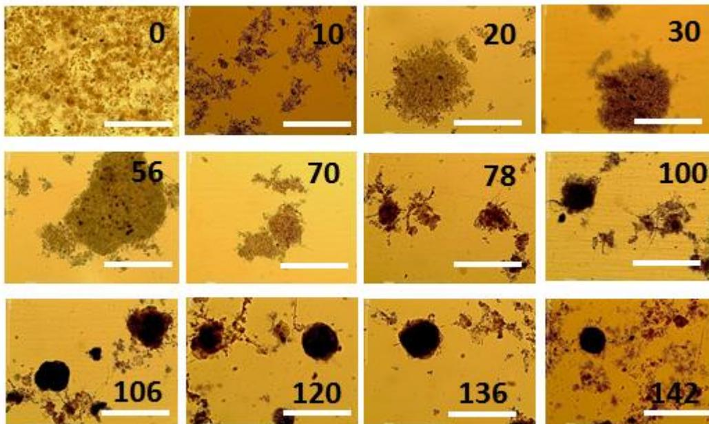
Figure 3: Morphological evolution of the sludge in the reactor. A number in each picture indicates the day of sampling. White scale bar represents 500µm.
