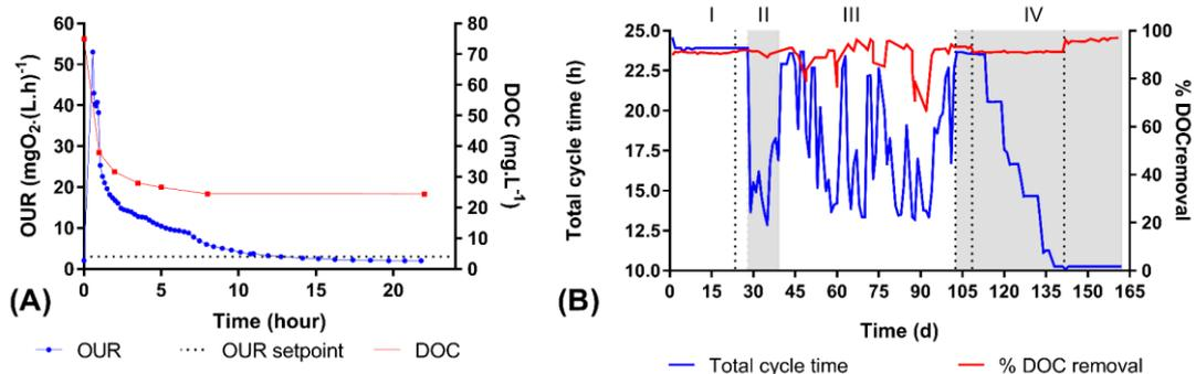
Figure 4: (A) Respirogram of the reactor at day 29, before starting stage II together with the DOC removal and the OUR set point for the endogenous aeration rate (B) evolution of the total cycle time and the DOC removal during the whole reactor operation. (Vertical dotted line represents a switch to a new influent batch) (note: in stage III, a new influent batch was used every day).
