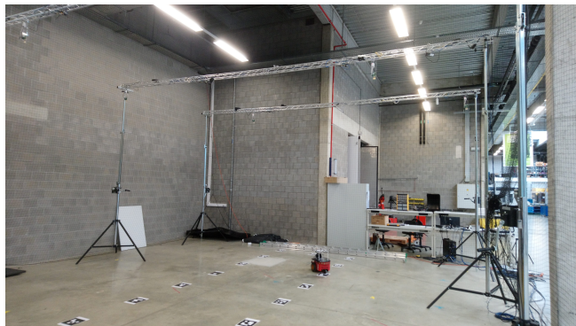
Fig. 3: Experimental setup. Depending on the experiment, the anchors are mounted on the fixed metallic trusses or on tripods further away from the testing area. The cameras providing optical ground-truth are mounted on the trusses and calibrated using ArUco markers at known positions on the floor.
