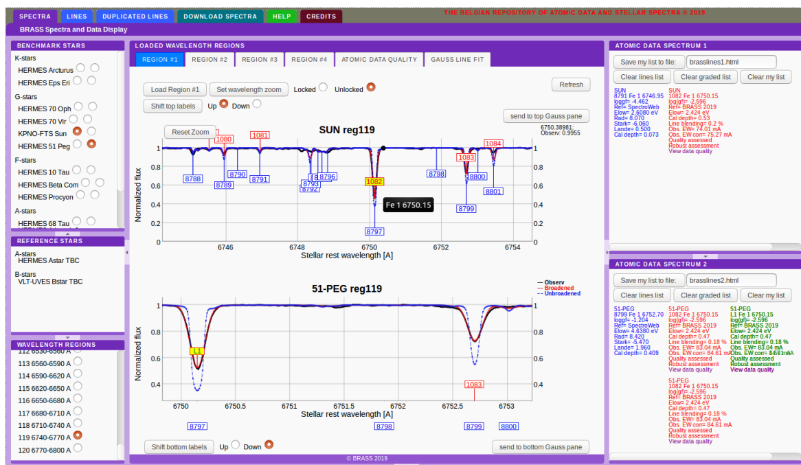
Figure 3. Screenshot of the SBDI for the solar FTS spectrum (central top panel) and the BRASS benchmark HERMES spectrum of the solar-like star 51 Peg (central bottom panel). The red and blue interactive labels mark identified absorption lines with atomic and line property data tables shown in the right-hand sub-panels. Atomic quality assessment pages are displayed under the central Atomic Data Quality tab by clicking on the View data quality link in the red or green line data tables.
