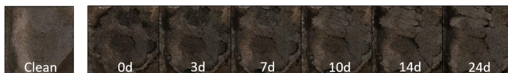
Figure 6.7. Subsequent digital images of soot degradation on a PFC photoanode coated with P25 when flushed with water vapour with f.l.t.r. a photoanode without soot, with soot before UV illumination, after 3, 7, 10, 14 and 24 days of UV illumination.
