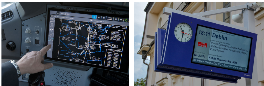
Figure 54 A display used in an airline cockpit displaying flight navigation maps (left) and a display on a train platform (right) support different content, but are identical in form. Pictures taken from Thales, 2019 and Dysten, 2020.
