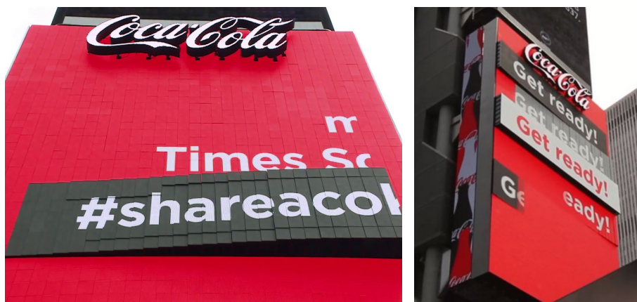
Figure 46 Coca Cola shape-changing display billboard. The actuated LED panels adapt their position to match the displayed graphical content. Pictures courtesy of Radius Displays.
