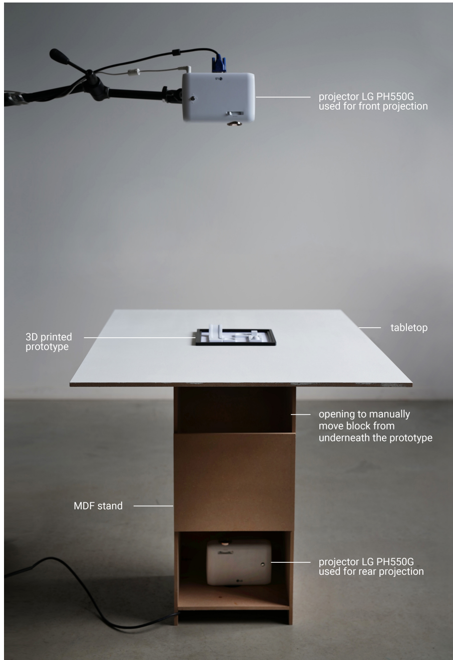
Figure 42 Picture of the projector setup consisting of a MDF stand and white painted tabletop that is constructed to hold the prototype and to position the projectors for filming the interaction routine.
