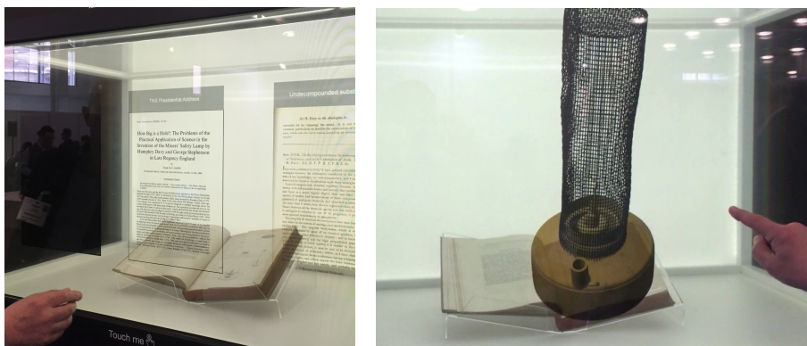
Figure 50 Transparent display used in a museum booth. In this particular example the user can look through a book by flicking through pages displayed on the transparent display and zooming in, without damaging the artefact (left). Next to flipping through the book's pages the visitor can interact with the virtual objects that are presented on the display (right) (CDS, n.d.).
