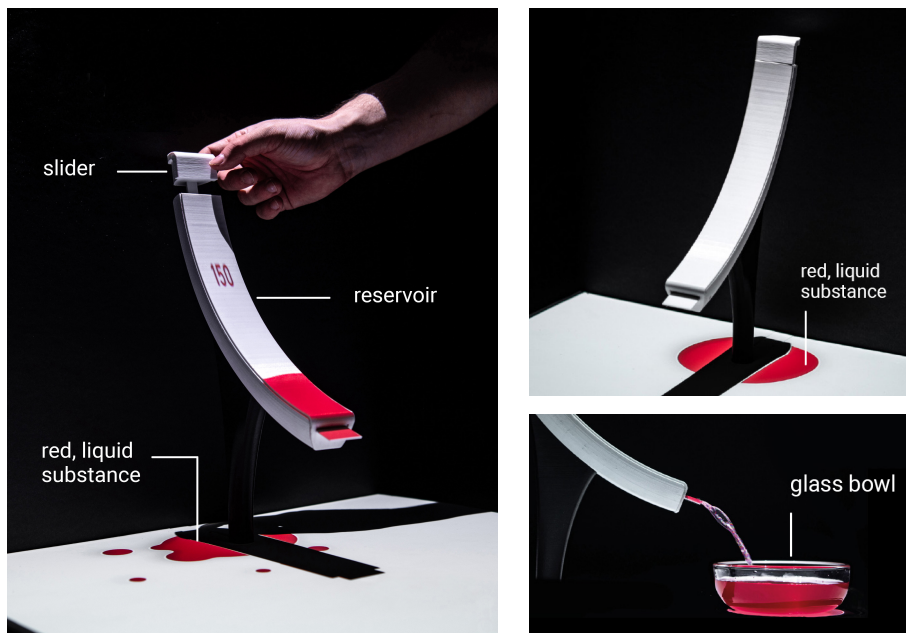
Figure 55 Presentation of the Furo prototype and its components. Left: user pulling the slider to fill the reservoir. Top right: the tap is in rest state. Red, liquid substance is displayed on the platform under the tap and shows that the tap is ready to be used. Bottom right: glass bowl being filled with the water from the reservoir.
