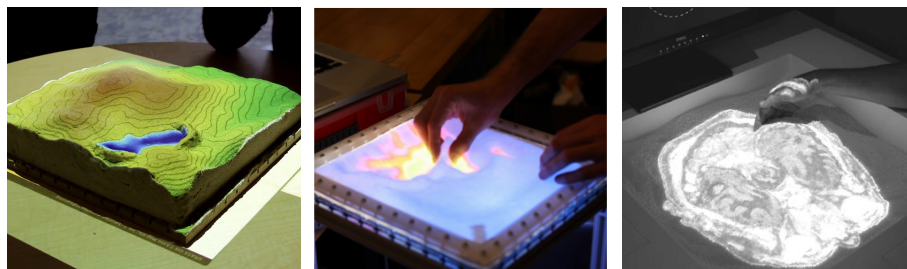
Figure 49 Left: the Tangible Landscape prototype allows to sculp a terrain in sand. Landscape elements like water and contours are graphically-augmented onto the prototype (Harmon, 2016). Centre: the Tunable Clay prototype is a square malleable display designed to mimic the malleability of clay that can be used to deform or sculpt the displayed graphical content (Follmer et al., 2012). Right: the Phoxel-Space prototype is used for medical imaging and can display non-planar images of a human brain scan (Ratti et al., 2004).
