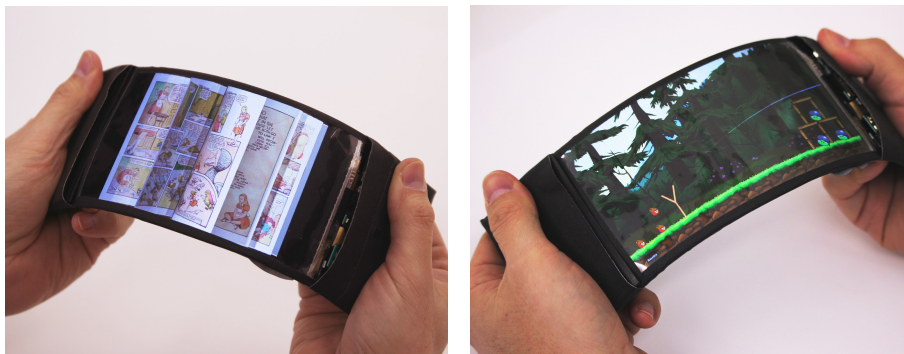
Figure 47 The pictures show two uses cases of the Reflex prototype. Left: user bending the prototype to move through the displayed document as if he/she is flipping through the pages of a book. Right: user bending the prototype to stretch a sling shot in the Angry Birds game. Pictures courtesy of Queen's University's Human Media Lab.
