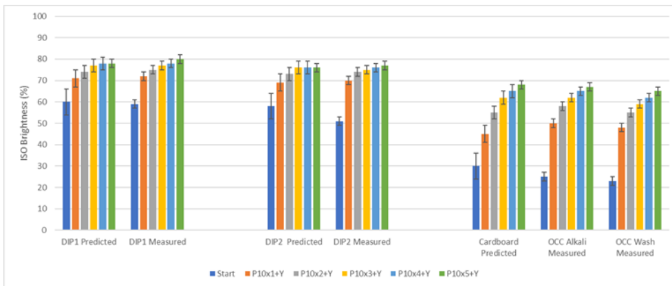
Figure 8 Comparison between measured values and predicted values during bleaching sequence P10+Y after correction
