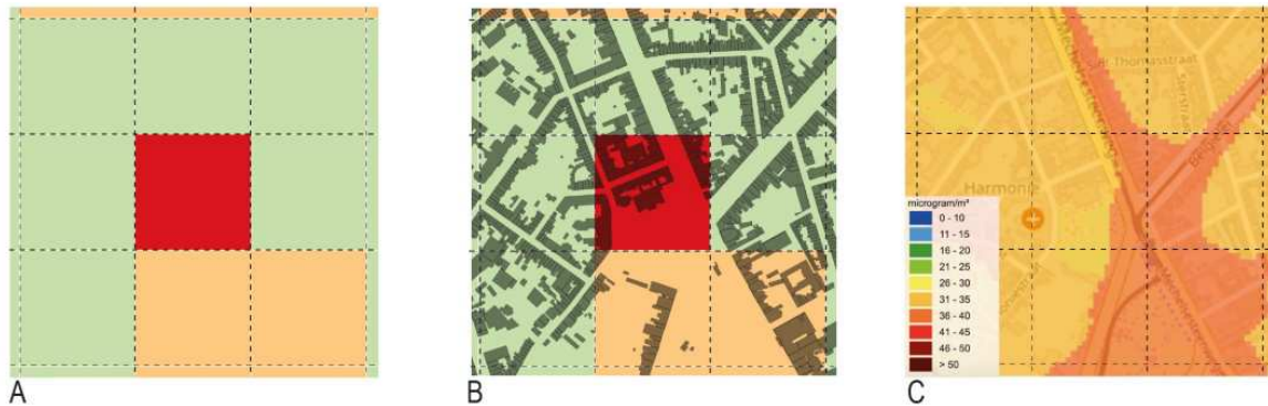
546 547 Fig. 13. Application of the potential increased exposure map for the Koning Albertpark in 548 Antwerp, with (A) the mapping of the potential increase exposure zones, (B) the 549 combination of the potential increased exposure zones and the urban fabric and (C) the 550 NO_2 pollution level model [45] 551
