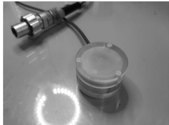
FIGURE 1 UTIC1 prototype with a distance between electrodes of 0.27 mm
