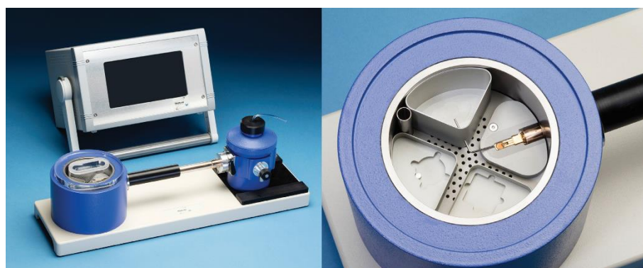
Figure 6.8 – Fischione model 2550 cryo-transfer tomography holder, with details on the recipient for liquid nitrogen to perform the grid transfer to the holder 300 .
