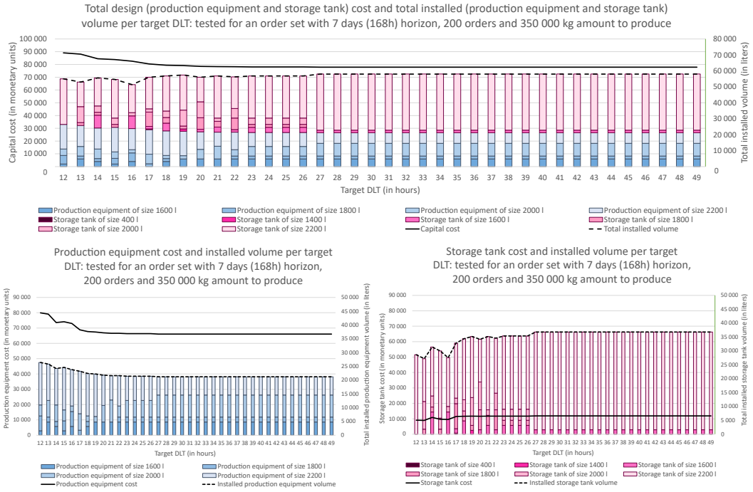
Figure 6: Above: Optimal capital cost and total installed volume of production equipment and storage tanks per target DLT for an order set comprising 200 orders, a total amount of 350 000 kg and an horizon of 7 days (168h) (order set 168) Below: cost and installed volume for production equipment and storage tanks separately
