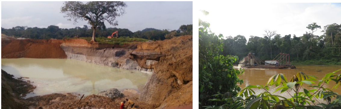
Figure 8. images of Chinese-led semi-industrial gold mining operations at the edge of Itombwe Nature Reserve in the village of Kitumba, Wamuzimu chiefdom. The site on the left is an open-pit mine excavated by mechanical diggers. On the right is a mechanised dredging operation in the Ulindi River.
