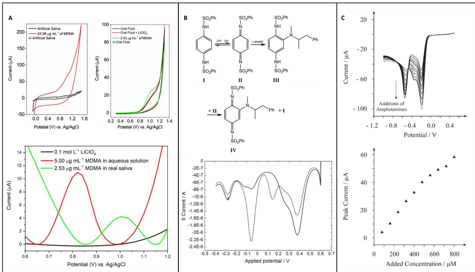
**Figure 2** Electrochemical strategies for the detection of ATS in oral fluid. A) SWV detection of MDMA at carbon paste electrode and SPCE.<sup>45</sup> Copyright 2020, Elsevier B.V. B)  $N,N'$ -(1,4-phenylene)-dibenzenesulfonamide mediated SWV detection of methamphetamine at SPCE.<sup>48</sup> Copyright 2016, Springer. Adapted. C) NQS-mediated detection of D-amphetamine sulphate.<sup>49</sup> Copyright 2006, WILEY-VCH Verlag GmbH & Co. KGaA.
