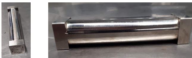
Figure 3-2 Thin Film applicator for bitumen
