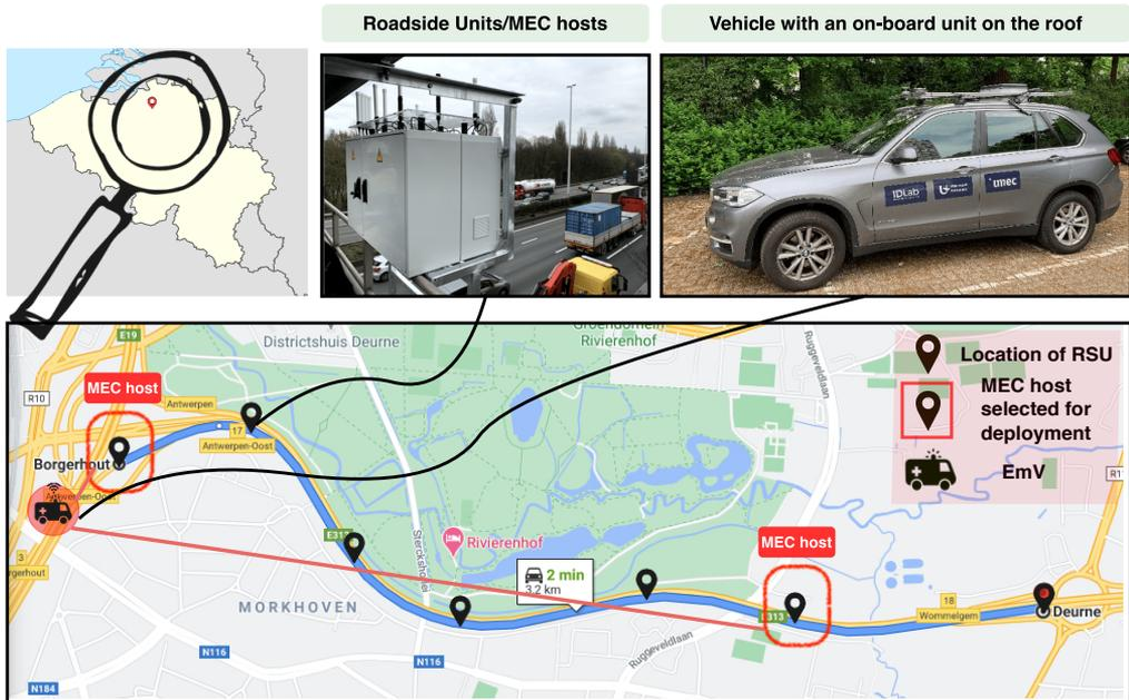
Figure 5.9: The experimental setup consisting of the vehicle, and the MEC hosts deployed on the E313 highway (Antwerp, Belgium).
