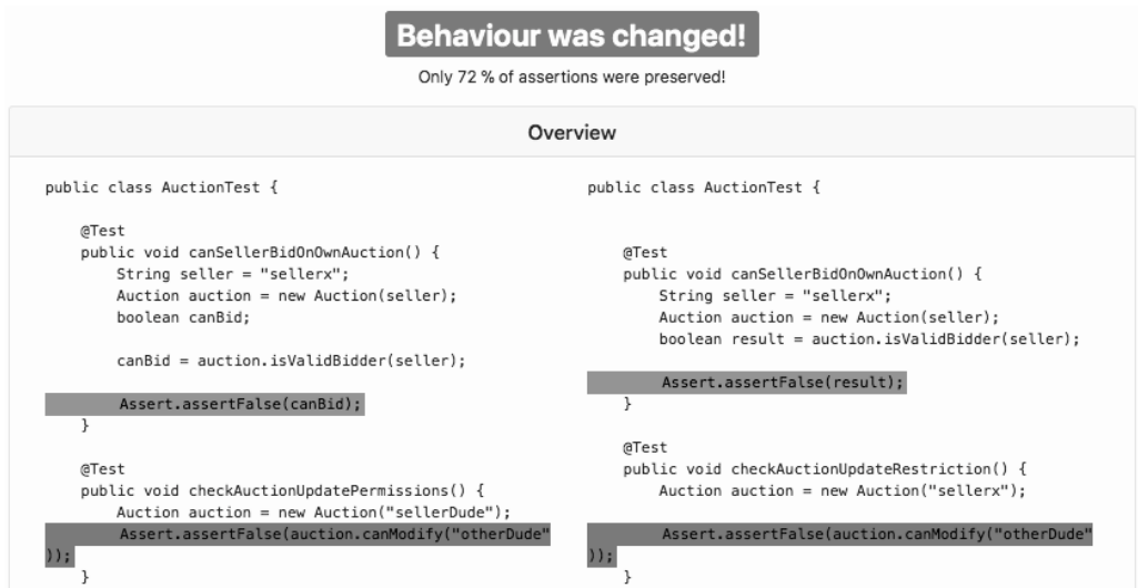
Figure 4.1: Example of a part of the T-CORE output when run on a behaviour changing refactor.
