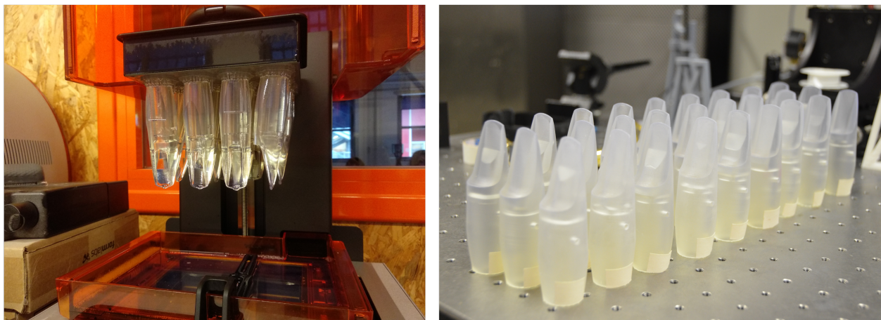
Figure 1: 3D printing mouthpieces (left), various mouthpiece designs used in the experiments (right).
