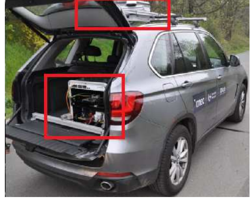
Fig. 7: The OBU Roof Unit placed on the vehicle roof and the OBU Car Unit placed inside of vehicle.
