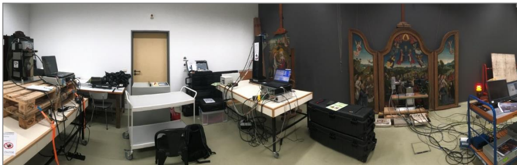
Figure 4.4-10 The three scanners in action during the 2019 MetOx scanning campaign. From left to right: MA-rFTIR, MA-XRF and MA-XRPD.
