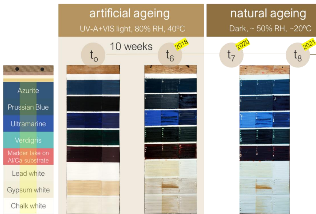
Figure 4.4-7 Mock-up stratigraphic oil paint systems with artificial and natural ageing conditions. Characterisation measurements were realized at different time intervals labelled t_0 to t_8 .
