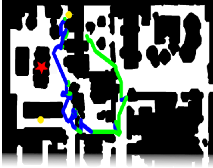
Figure 7.8: An example trajectory of the agent in a scan of The Beacon office building. The red star is the new goal, while the prior goals are marked with a yellow circle.
