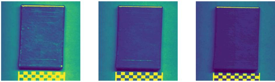
Figure 7.15: Three frames from the temporal matrix (Left) Frame 1; (Middle) Frame 50; (Right) Frame 100. Notice that due to heterogeneous illumination from the UV light source, the different frames of the temporal matrix show a different brightness value.
