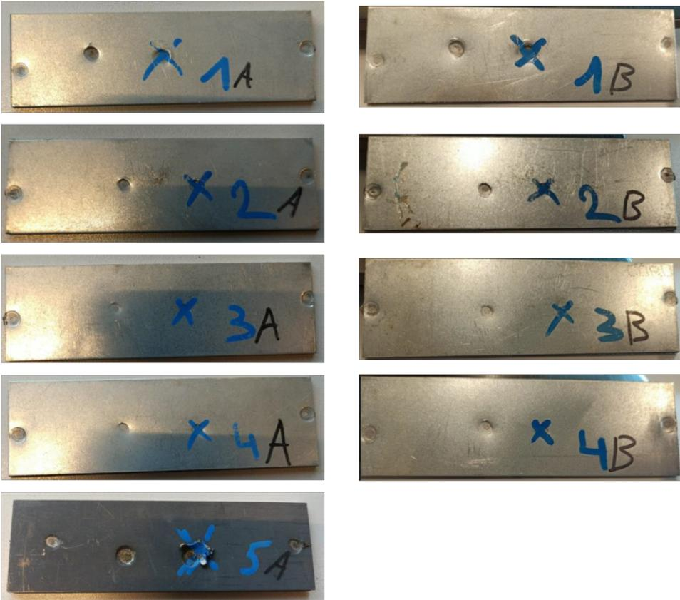
Figure 2.1: Nine samples, divided into two series. The A-series consists of four samples with a thickness of 2.5 mm (1-4) and sample 5A is 3.15 mm thick. The B-series only consists of four samples with a thickness of 2.5 mm. The spot weld highlighted by the blue cross is the inspected spot weld for each sample.
