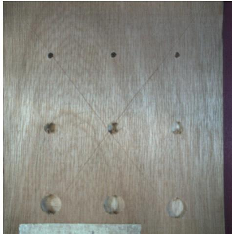
Figure 7.10: RGB image the inspected bottom wooden sample, so the defects are visible. The dimensions are following: 160x100x5.8 mm.
