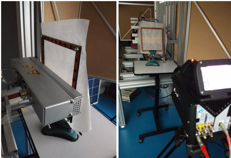
Figure 3.9: In the left picture, the MES-heater is visible in the measurement setup. The setup consists of the line heating source, a baking paper clamped between two wooden frames and the FLIR X6540sc infrared camera. The baking paper is used to investigate the heated area of the sample in transmission mode. The baking paper was placed at a distance of 1.5 cm from the bottom of the line heater as recommended in the datasheet.
