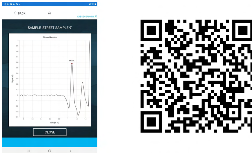
Figure 4.5: Screenshot of the processed voltammogram of street sample 9 measured in ACE pH 5 buffer, as shown in the mobile application (left). The diagnostic peak of MDMA around 1.11 V is clearly visible. Other screenshots of the mobile application are shown in Figure S4.7. Scanning the QR code will redirect you to a video that demonstrates the final sensor (right).
