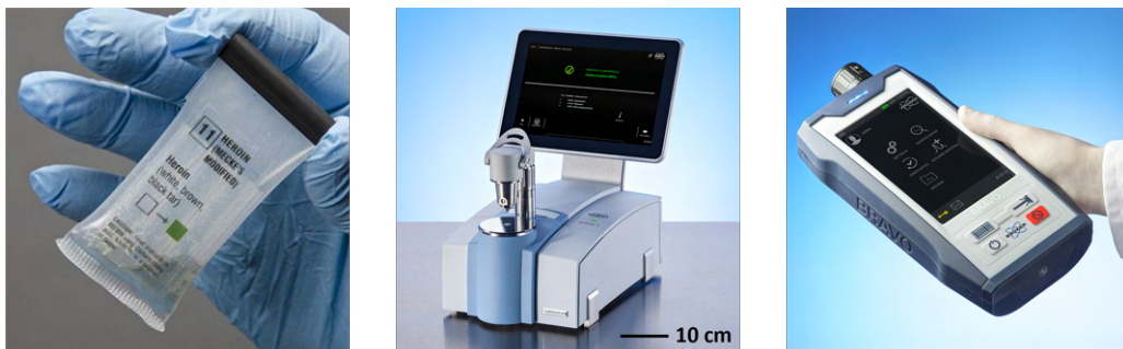
Figure 1.4: Colorimetric tests and portable spectroscopic techniques dominate the illicit drug on-site detection field. From left to right: commercial color test for heroin detection, portable ATR-FTIR device and portable Raman spectroscopy device. The latter two are used in this thesis for competitive analysis.
