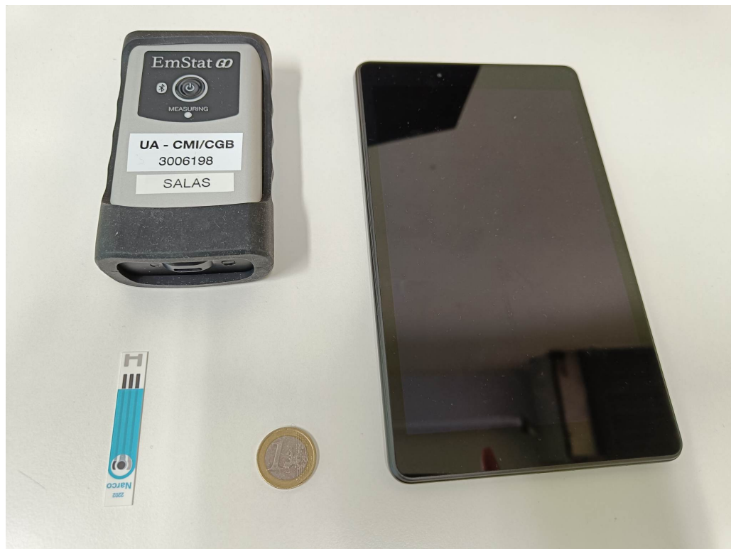
Figure 2.3: Overview of the SPEs (bottom left), potentiostat (top left) and tablet (right) mainly used during this thesis, with a 1 euro coin for reference.
