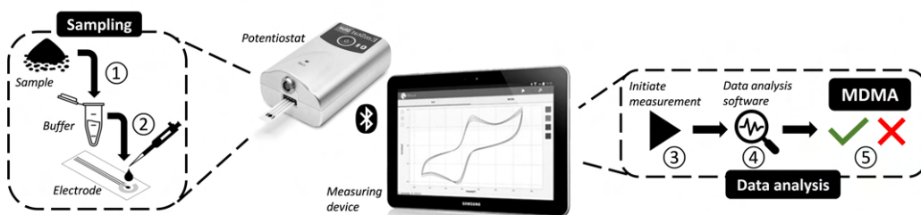
Figure 2.4: Blueprint of voltammetric illicit drug sensor, displaying the different steps of a measurement. First, a few milligrams of a sample is dissolved in a buffer solution (1). Subsequently, a few droplets of the resulting solution are placed on the surface of a SPE (2). This SPE is inserted in a potentiostat, which is wirelessly connected to a measurement device such as a laptop or smartphone. Software is installed on this measuring device that allows to start a voltammetric measurement with a single click (3). After the measurement is done, data analysis software can be included which automatically converts the voltammetric output into a clear-cut interpretation thereof (4,5).
