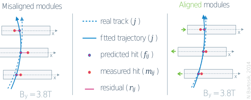
Figure A.1: Schematic view of a charged particle traversing detector layers (dotted blue line). Fitted particle trajectory (solid blue line) is shown in situation with misaligned tracker modules (left) as compared to corrected tracker geometry (right). Residual distance between predicted trajectory and actual detector hits (solid red line) is minimal in case of perfectly aligned tracker. Source [163].
