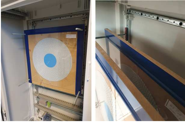
Fig. 3. The coils for the inductive WPT transfer installed in the BIPV housing (left), indicating the easily adjustable distance between transmitter and receiver coil (right).
