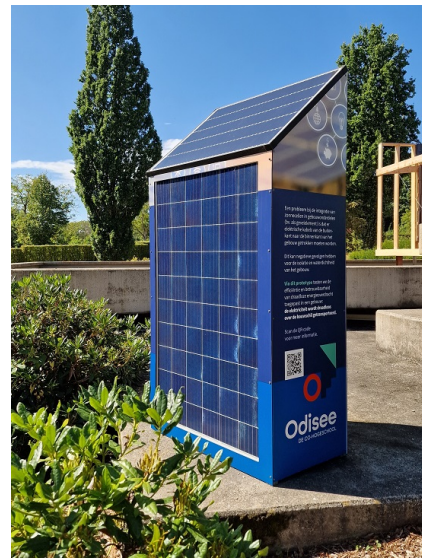
Fig. 1. Housing of the BIPV demonstrator: power generated by the vertical photovoltaic panel is transferred wirelessly via coupled coils to a load inside the housing. The roof solar panel is aesthetic and not electrically connected.
