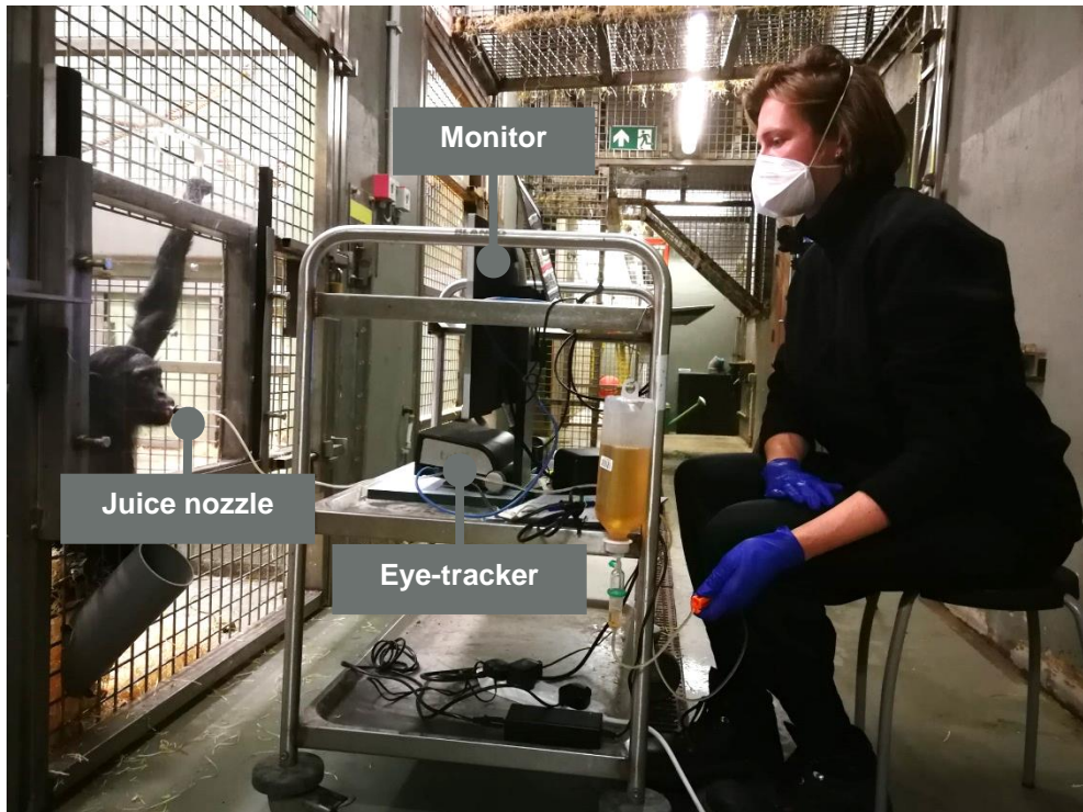
Figure 3.1: Overview of the eye-tracking setup
