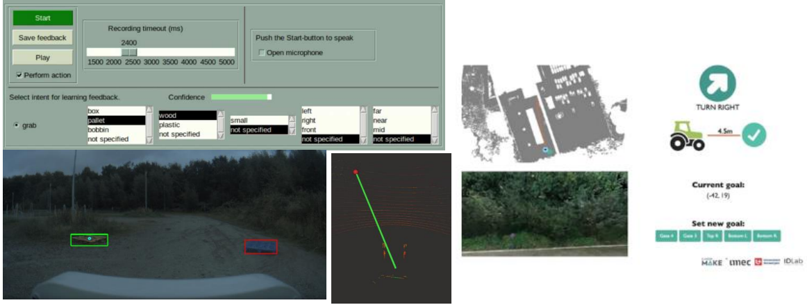
Figure 11. Snapshot of the demonstrator of the AGV Multi-modal AI framework: (top left), the Speech model interface, (bottom left), the Vision model interface, (right), the Navigation digital twin interface, (bottom middle), the estimated trajectory between the AGV.
