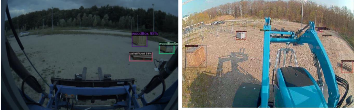
Figure 6. (left) all objects are correctly classified, (right) some objects are not detected.
