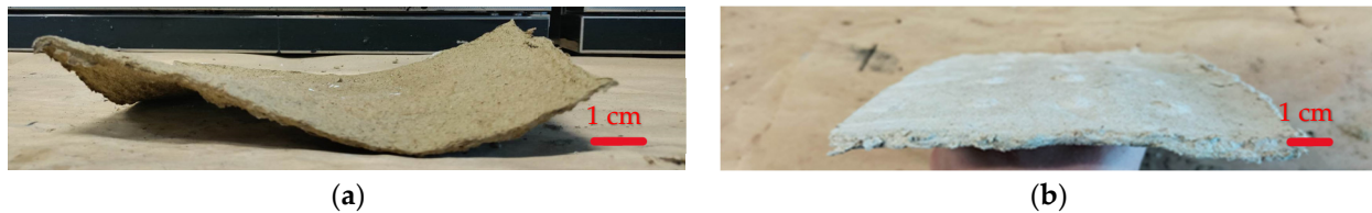
Figure 5. (a) Sample '90/10' curved after drying period; (b) sample '90/10-M60' preserved shape after drying period.
