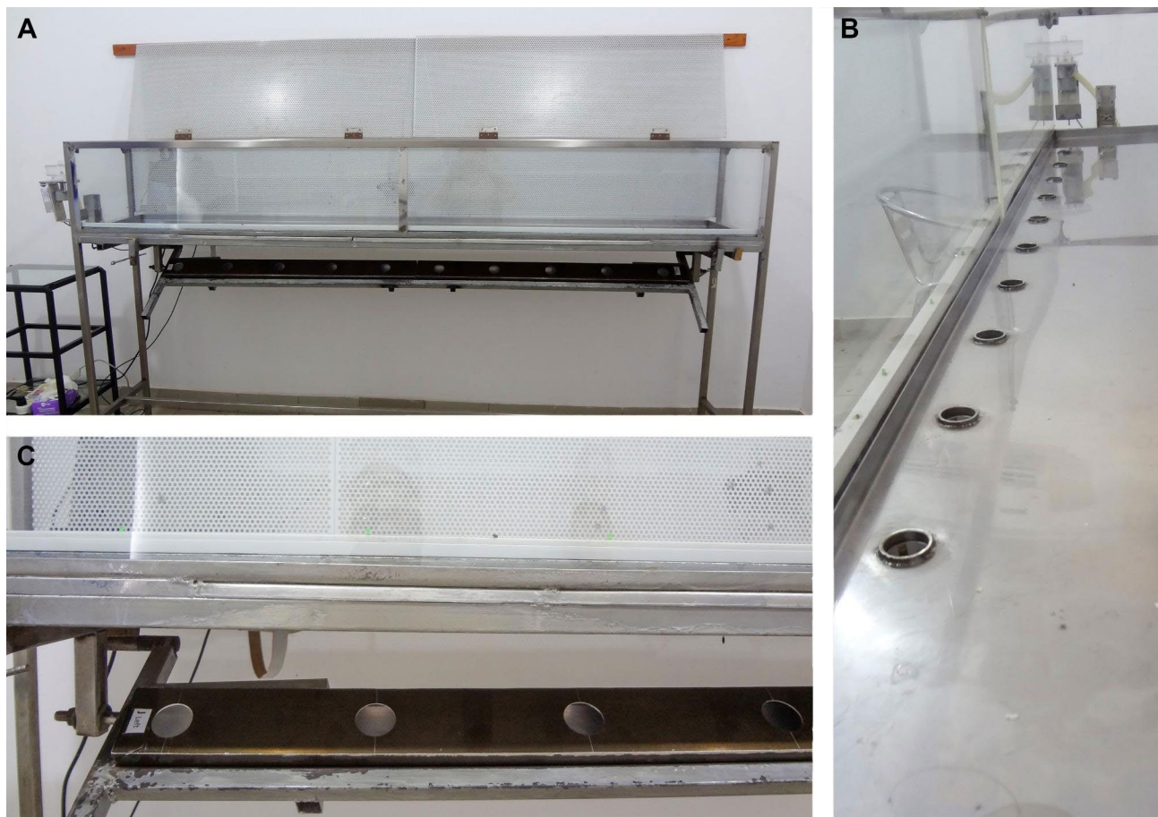
Fig. 4 Photographs of the front (A) and side (B) view of the rectilinear scent evaluation apparatus. Cups containing culture sample solutions were placed within bars (C) that could be swung up and locked to position the sample beneath the holes along the floor of the apparatus. Rats were trained to walk from one side (beginning near the food pellet dispenser shown to the left in A) to the other, sniffing each sample in sequence as solenoids below the floor slid a metal plate to uncover each sample. Light emitting diodes (LEDs; pictured to the left of the floor holes along the white rail in B) illuminated when a hole was uncovered. Infrared emitting photobeams and sensors positioned within each hole registered when and for how long the rat inserted its nose. Flavored food pellets were automatically dispensed when the rat held its nose within a hole containing a Brucella -positive sample for the pre-scribed duration
