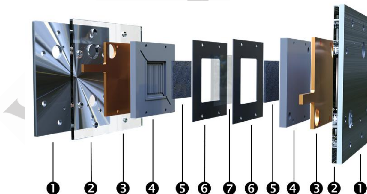
Figure 5. Exploded view of the VFB components: aluminium backplates (1), PMMA insulator plates (2), copper current collectors (3), impervious graphite monopolar plates (4) providing parallel flow channels and a compartment for the graphite felt electrodes (5), gaskets (6) and Fumasep FAP-450 membrane (7).
