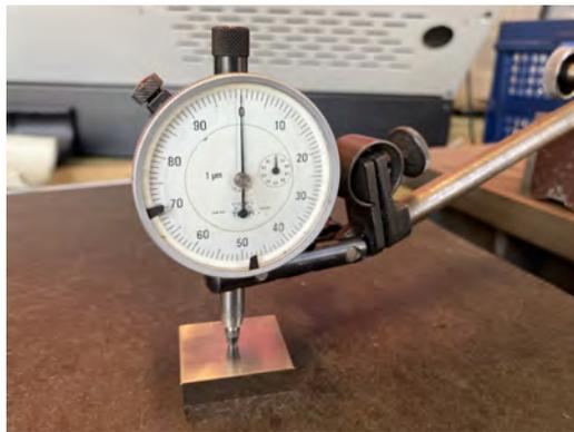
Figure 2.18: Measurement of the flatness of the ground side of a gauge block using a dial indicator to serve as flat calibration object.
