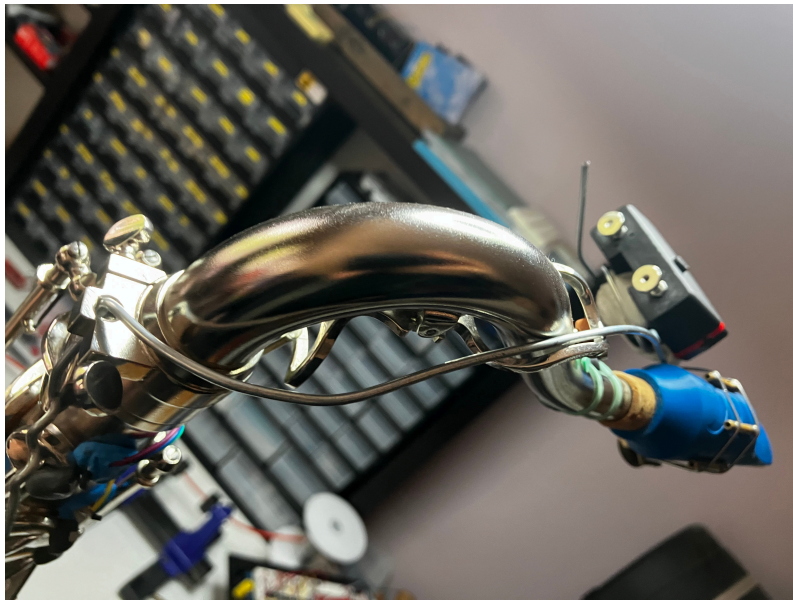
Using the marching band music stand adapter screw for connecting the digital mouthpiece (Photon)
