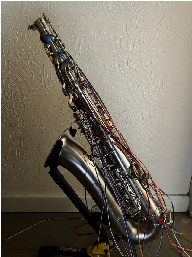
Sensors mounted on the body of the saxophone
