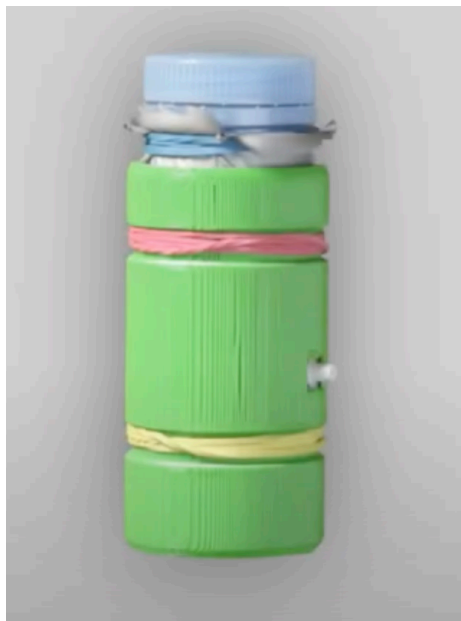
KontinuumLab's nifty low cost DIY breathcontroller
