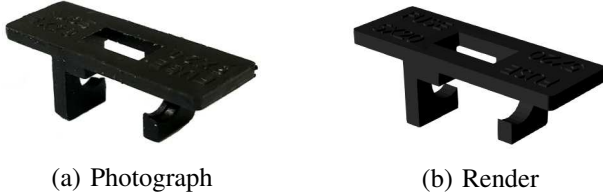
Fig. 3. The fuse cover sample: (a) shows a photograph of the real sample and (b) shows a render of the CAD model.
