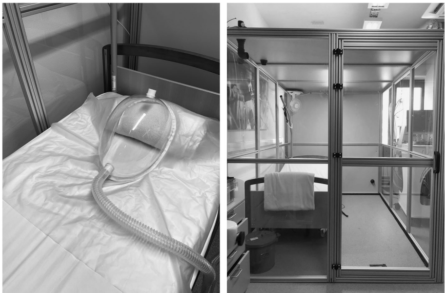
Fig. 1 Modalities used for measuring energy expenditure. Left: Ventilated hood; Right: Basic respiratory room
