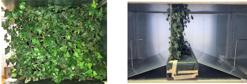
Fig. 2 Left: Detailed picture of H. helix facing the air stream in the wind tunnel setup, illustrating the realistic arrangement of the climber (in terms of coverage and growth depth). Right: the planter grown with H. helix in middle of the test section with ramps guiding the air flow at both sides.
