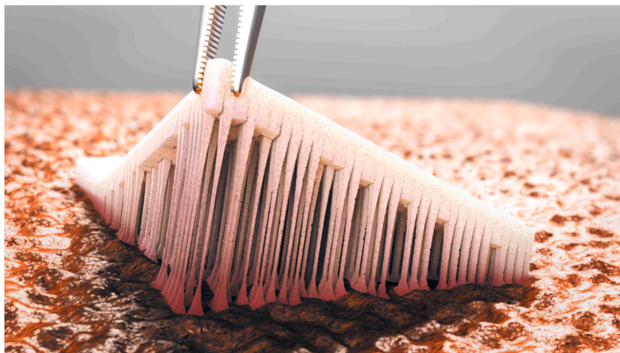
Fig. 1. TenaTac has a uniquely modified surface that consists of over 1000 columns (each 3–4 mm high and 1.5 mm wide) which increase surface area. In addition, the columns can also each interdigitate with the irregular surface of bleeding tissues, thereby greatly increasing surface contact. In addition, because the patch is made of gelatin, each column acts as an elastic attachment to the surface helping to resist any applied shear force.
