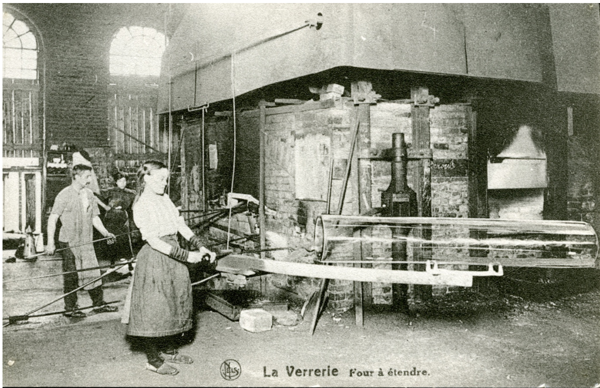
Figure 15: Introduction of glass cylinders into the annealer (presumably Biévez-annealer)
