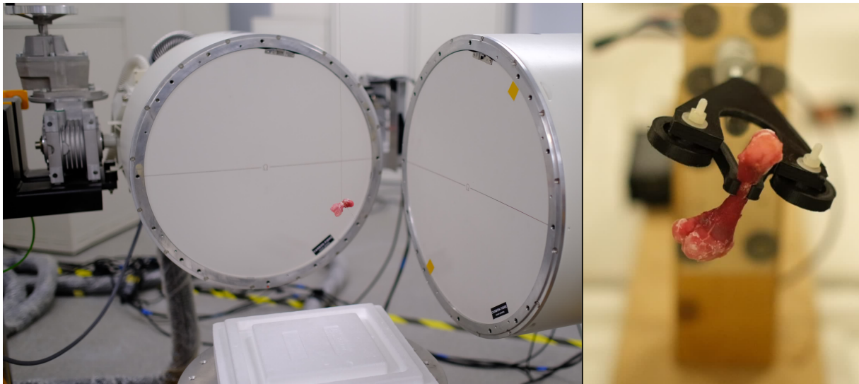
Figure 7.4: The "flying femur" experiment: an excised piglet femur used in XROMM experiments as an allegory of reductionism. Left: the femur oscillating on a pendulum. Right: installation with a motor capable of moving the femur in a realistic way.
