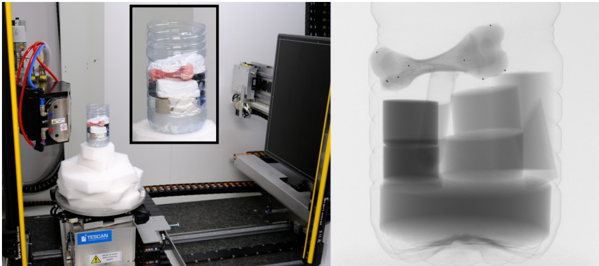
Figure 7.3: Experimental Setup. A piglet femur was excised and marked with metal bead markers. Together with various calibration objects, the sample was fixed (“mounted”) in a PET bottle to fit into the cylindrical scan volume of the FleXCT scanner of the University of Antwerp. The image on the left shows the sample mount, magnified on the inset. On the right is one CT projection of the sample, with the femur with markers clearly visible on top.
