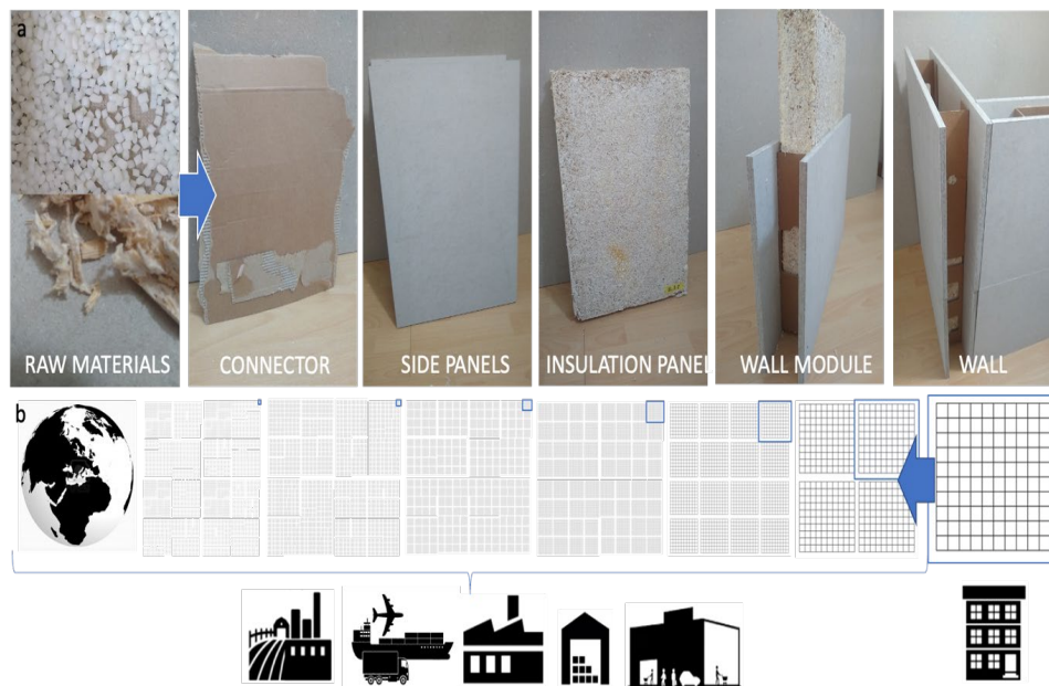
Figure 6. Integrated view on parts and spatial distribution. 6a: From raw materials to wall configuration, and 6b: from building scale to global supply network.
