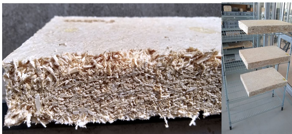
Figure 2. Mycelium Fiber Insulation board drying in the lab.
