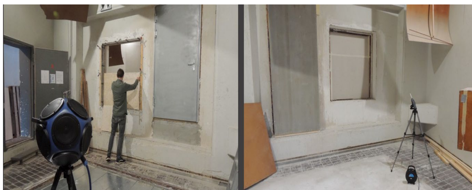
Figure 4. Set-up of sound insulation test: EN-EN-ISO 10140-2.
