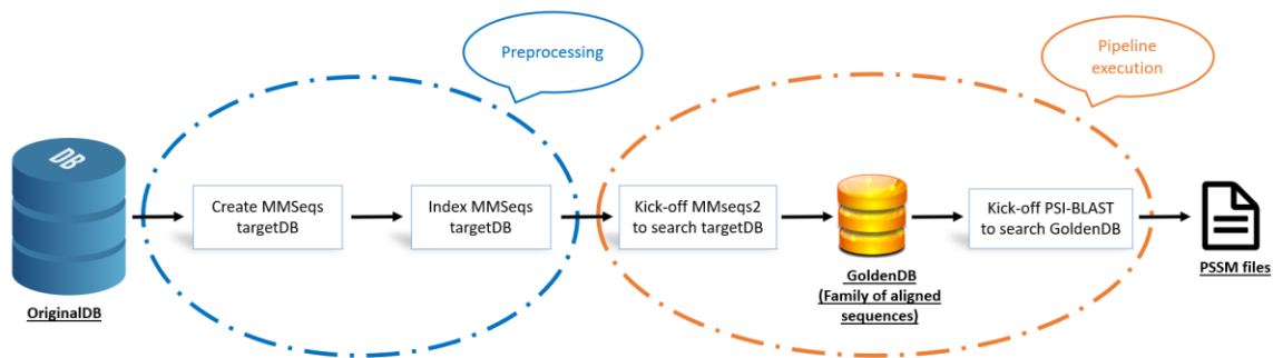
Figure 1: EPSAPG high-level architecture. The high-level architecture consists of two main parts: a preprocessing step, blue section, and a pipeline execution step, orange section. The preprocessing procedure compiles an MMseqs database, named targetDB, from the FASTA file of the original database to be searched. From the targetDB, a large index table is constructed that later will be used by the pipeline for a fast query alignment. The preprocessing step is crucial for a faster and reusable index table in future runs.
