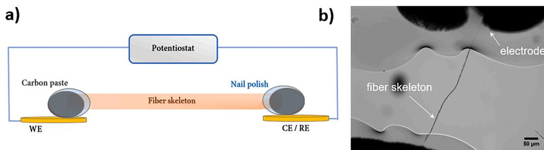
**Fig. 3.** a) Schematic of measurements of an individual fiber skeleton. WE – working electrode, CE – counter electrode, RE – reference electrode. b) Micrograph of an individual fiber skeleton stretched between electrical contacts (carbon pads waterproofed by nail polish).
