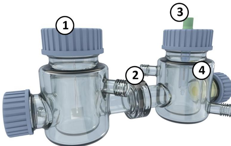
**Figure 3.1.** Electrochemical set-up designed for the long-term electrolysis: (1) Pt counter electrode (CE), in the cathodic compartment; (2) Nafion membrane; (3) reference electrode (RE) and (4) working electrode (WE), both in the anodic compartment.
