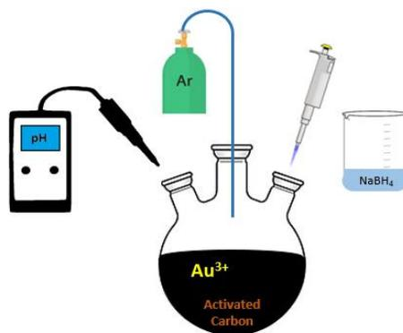
**Figure 5.1.** Schematic representation of the synthesis of AuNPs/C catalyst by impregnation.
