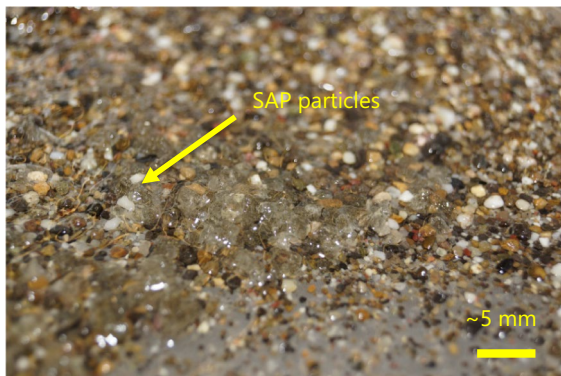
Fig. 1 SAP particles and sand left on the sieve after Step 3 of Method A. Based on such outcome, the presence of SAP in fresh concrete is confirmed qualitatively
