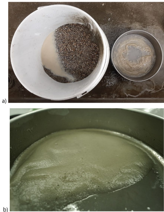
Fig. 2 a Separation of concrete by adding excess water according to Test 1, Method B; b SAP collected on the sieve after the separation procedure
