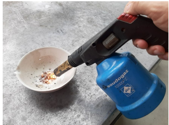
Fig. 3 Burning out of SAP particles with a gas torch
